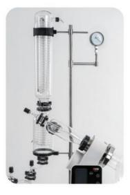
**Two-section vertical** triple coil condenser
